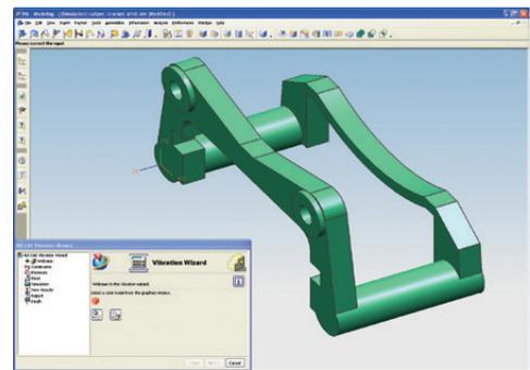
analysis processes. For each solid body component, users are prompted to assign a material specification, constrain the part, apply a load, automatically mesh the 3D geometry, and run the analysis using NX Nastran® software. With the NX Stress Wizard, users can review the structural performance image to ensure that the yield
