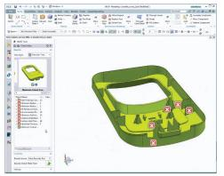
ibility of the designs, increase the operational life of the part and reduce manufacturing costs. Some of the important rules supported for castings checks include fillet radius, surface finish for machined faces, uniform wall thickness, mold wall thickness, wall thickness variation, draft angle and undercut detection.
