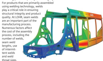
However, these factors also impact how the structure behaves dynamically and its affect on fatigue life.
