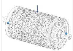
Steel rollers that help separate liquid and solid materials in manure were breaking during physical prototyping. Engineers suspected the honeycomb-shaped holes contained sharp edges that caused cracks. Using Solid Edge Simulation to test round holes showed better results; the resulting design proved to be much stronger and did not crack. The final model was created with Solid Edge.
