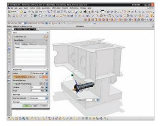
Synchronous technology quickly adapts assemblies and fixtures to accommodate new parts.
