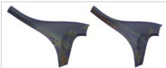
FIG. 2 The part in CAD can have the manufacturing process defined, refined and simulated to determine the best method with which to produce the part and how best to meet the analyst's desired fiber orientations. These two images demonstrate two different methods used for hand lay-up and the affect each had on the fiber orientations in blue, yellow and red. Yellow and red show deformations, where red indicates actual wrinkling of material.
