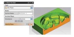
You can examine the part and the workpiece by viewing a cross section.
