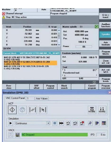
Virtual Machine uses the genuine Siemens control software with a complete operating panel display to drive the machine tool simulation.
