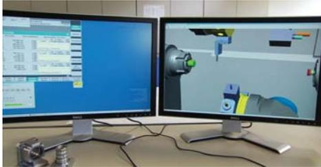
*You can validate NC programs on a virtual machine tool.*
