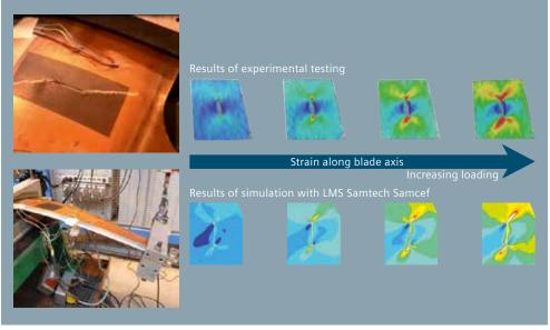
Correlation between LMS Samtech Samcef and test results showing damage on a helicopter blade. Images courtesy of Airbus Group Innovations.
