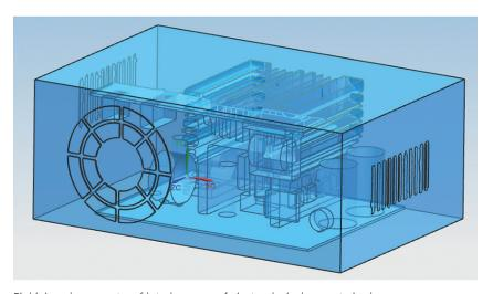
Fluid domain geometry of interior space of electronic device created using surface wrapping.
